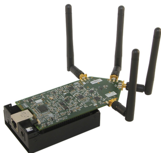
Figure 1: RF Ranging Basestation with Carrier-Phase and Angle-of-Arrival capabilities.
