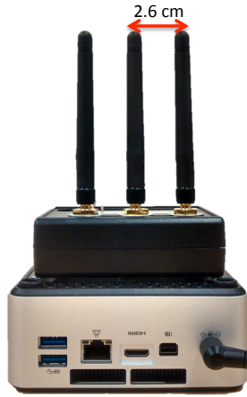
Figure 1: Access point with three antennas using Intel 5300 WiFi NIC embedded into Intel NUC (placed below the antenna array).
