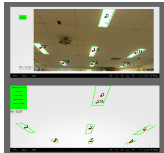
Fig. 1. An example of landmarks tracking registration which allows us to perform accurate indoor navigation using standard emitting lights.
