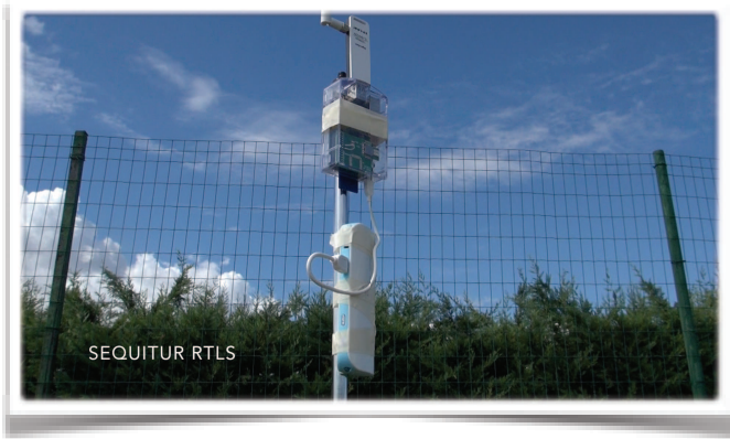
Fig. 1. Example of battery-powered SEQUITURE node.
