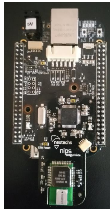
Power Over Ethernet NIPS Node (size 11 x 5.5 cm)
