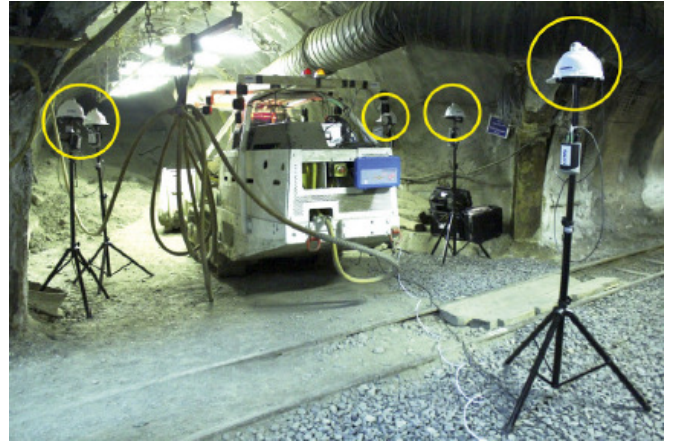
Fig. 2. Stationary measurement setup. The loudspeakers were mounted on a construction of wooden rails. The hard hats (circle marks), and mobile tags were mounted on supporting stands. (from [1])
