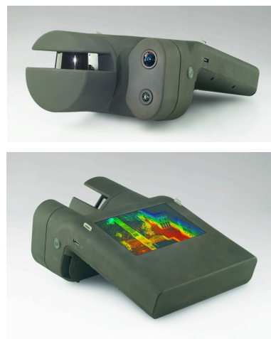
Fig. 1. Real Earth Contour is equipped with a spinning line scanner, a fisheye camera for state estimation, an HD color camera for point cloud colorization, an embedded i7 computer, and a touch-screen monitor.
