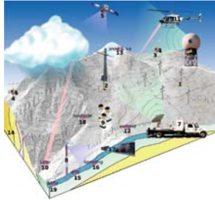
FIGURE 1. A typical data source context for next-generation environmental science, with a heterogeneous sensor deployment that includes (1) mobile stations, (2) high-resolution conventional weather stations, (3) full-size snow/weather stations, (4) external weather stations, (5) satellite imagery, (6) weather radar, (7) mobile weather radar, (8) stream observations, (9) citizen-supplied observations, (10) ground LIDAR, (11) aerial LIDAR, (12) nitrogen/methane measures, (13) snow hydrology and avalanche probes, (14) seismic probes, (15) distributed optical fiber temperature sensing, (16) water quality sampling, (17) stream gauging stations, (18) rapid mass movements research, (19) runoff stations, and (20) soil research.
