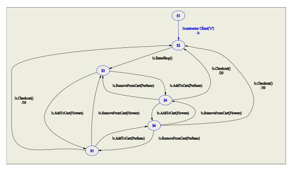
From an FSM as shown above we generate test sequences using the well-known traversal techniques (we use a variation of [5]). For the shown FSM we get a single traversal with 19 steps.
