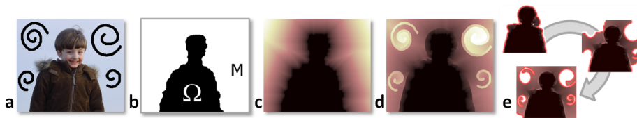
Fig. 1. \mathcal{O}(N) geodesic distance transform algorithms. (a) Original image, I ; (b) Input mask M with “object” \Omega . (c) Distance D(\mathbf{x}; M, \nabla I) from \Omega (with \gamma = 0 in (1)); (d) Geodesic distance from object ( \gamma > 0 ) computed with the raster scan algorithm in [18] (two complete raster-scan passes suffice). Note the large jump in the distance D in correspondence with strong edges. (e) Different stages of front propagation of the algorithm in [19], eventually leading to a geodesic distance similar to the one in (d).
