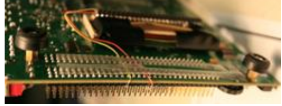
Figure 12: Pin hijacking platform
