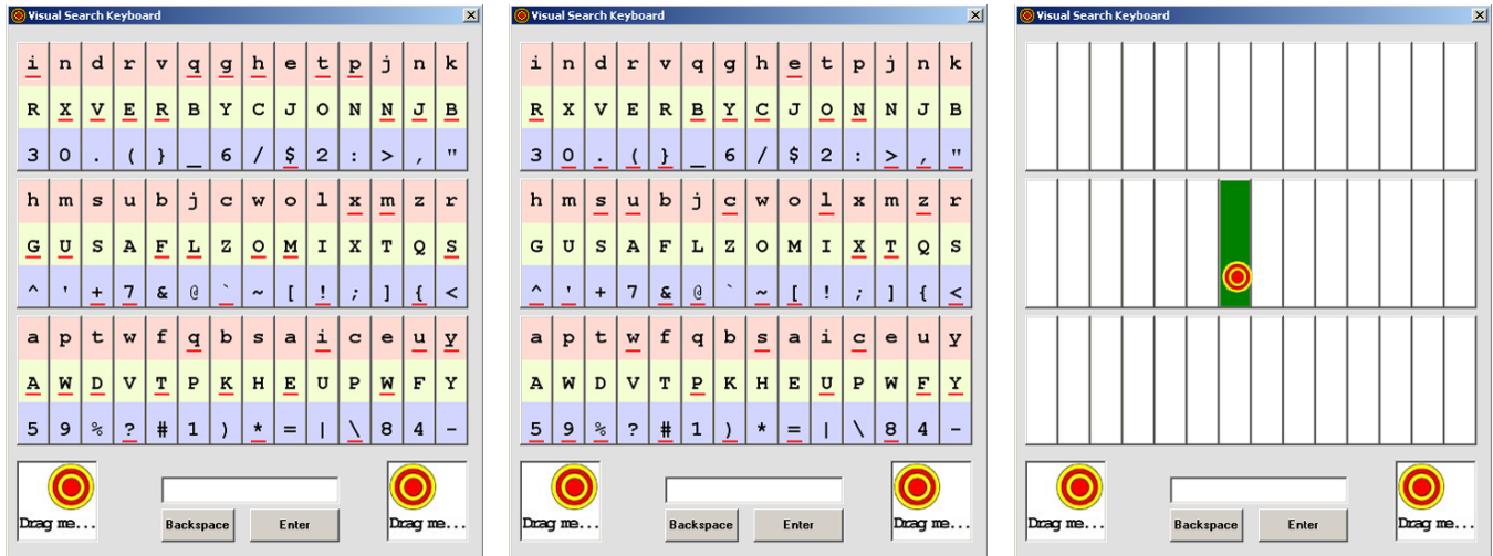
Figure 2: For example, user trying to type a “c” ( left ) searches Spy-Resistant Keyboard for the letter, finds it on the seventh Tile in the second row, ( center ) taps the Interactor once to shift the red underline to the “c” (all keys change shift state with each tap), and then ( right ) drags the Interactor to the appropriate Tile. It is very hard for an observer to reconstruct what has been typed.
