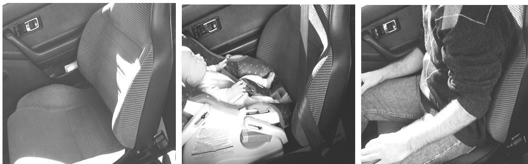
Figure 1: Empty, infant, and occupied seats as seen by camera inside vehicle. Airbag should not deploy on empty nor infant seat.
