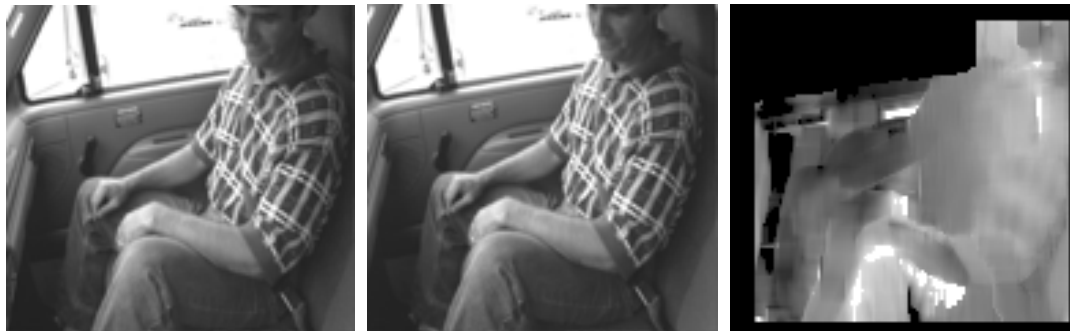
Figure 6: Stereo (left/right) images taken inside test vehicle. Rightmost image shows computed disparity, with lighter points having more disparity.
