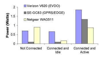
Figure 2: Power measurements of 1xEVDO, GPRS/EDGE and Wi-Fi interfaces for different scenarios. The "Connected and Active" measurements show the power when transmitting 32 Kbps of VoIP traffic over UDP. Note that when active, VoIP over Wi-Fi consumes the least amount of battery power.
