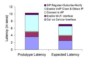
**Figure 9:** Breakdown of various steps of the Cell2Notify protocol in call-setup latency. The right bar shows the expected latency with our proposed optimizations. Even without optimizations, the extra delay is around ten seconds, which is less than two rings.
