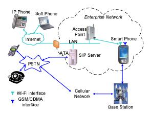
**Figure 1:** A typical enterprise VoIP deployment. Outside callers can either make VoIP calls over the Internet or over the PSTN line. The SIP server uses an Analog Telephony Adapter (ATA) to translate the call from PSTN to IP and vice-versa.
