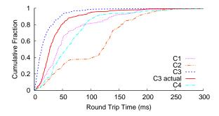
Figure 12: This figure shows the cumulative distribution of the optimal round trip time (RTT) to the instances deployed on a cloud provider from 260 global vantage points. For  $C_3$  we also show the actual RTT from a vantage point to the instance returned by the cloud's DNS load balancing.
