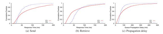
Figure 9: The cumulative distributions of the response time to send or retrieve a message from a queue, and the propagation delay of a queue.
