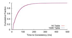
Figure 5: The cumulative distribution of the time to consistency for  $C_1$ 's table service.
