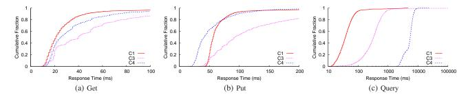
Figure 4: The cumulative distribution of the response time when using the large table with 100K entries. Note that for the query operation, the x-axis is in a logarithmic scale, due to the significant performance gaps between different services.
