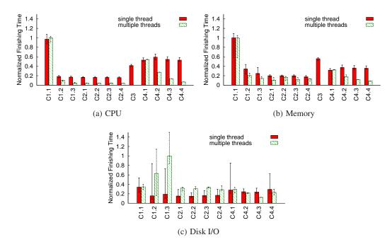
Figure 1: The finishing time of benchmark tasks on various cloud instances. The time values are normalized using the longest finishing time to emphasize each provider's relative performance. We show both single-threaded and multi-threaded results. The multi-threaded and I/O results are missing for  $C_3$  because it does not support multi-threading or accessing the local disk.
