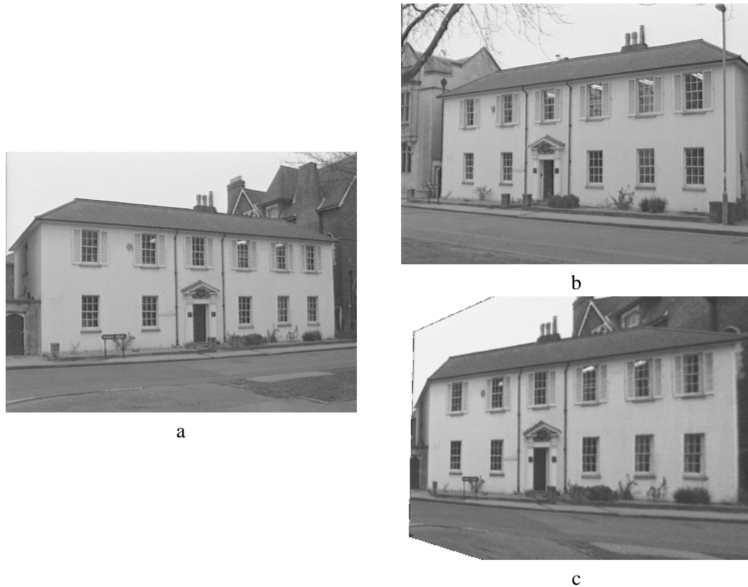
Figure 4.10: Warping planes between images: (a,b) original images from two different points of view; Crystallography labs, Oxford. (c) first image warped onto the second by the inter-image homography.
