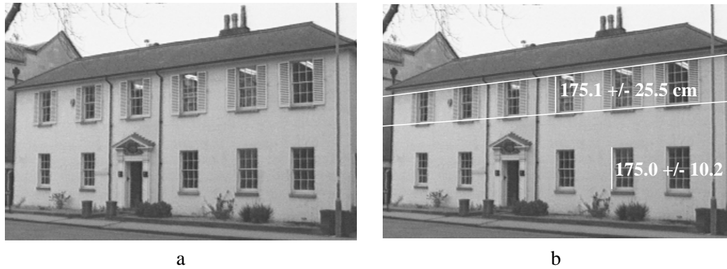
Figure 1.5: Measuring distances and estimating their accuracy: (a) original image, a photograph of the facade of the Crystallography Laboratories, Oxford; (b) the height of different windows has been computed and the accuracy estimated.
