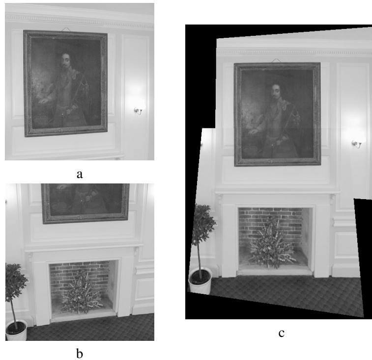
Figure 1.7: Mosaicing two images: (a) and (b) two images of The Queen's College MCR in Oxford; (c) mosaiced image; the images have been perspective-corrected and stitched together.
