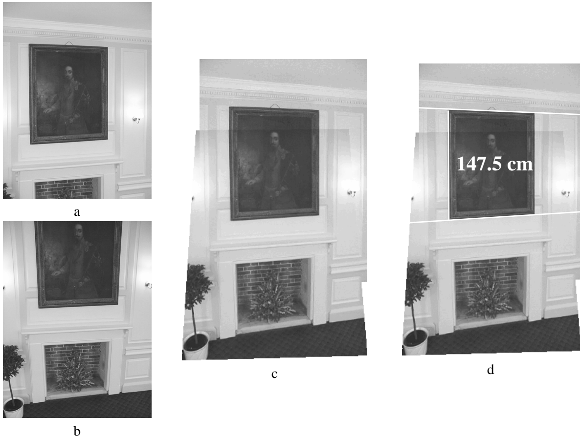
Figure 4.16: Mosaicing two images: (a) and (b) original images of The Queen’s College MCR in Oxford; the two images are taken from the same viewpoint (no parallax effect); (c) mosaic image; (d) mosaic with measurements superimposed.
