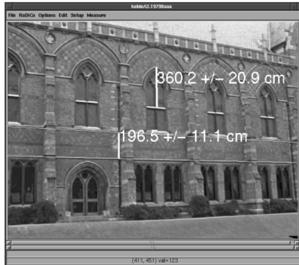
Figure 4.7: Graphical User Interface: example of the measurement stage. It involves an easy-to-use graphical interface; the user is only required to select the two end points of the segment to measure.
