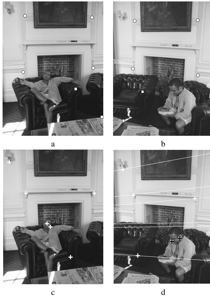
Figure 6.4: Consistency with the epipolar geometry: (a) and (b) left and right view of an indoor scene in which the person has changed his position. Four pairs of corresponding points on the wall (white circles) have been used to compute the inter-image homography. Two pairs of corresponding points not on the wall plane (white boxes) have been used to compute the parallax geometry (points \mathbf{p} , \mathbf{p}' , \mathbf{q} and \mathbf{q}' in text). (c) and (d) some points have been selected on the left image (white crosses, point \mathbf{x} in text) and the corresponding epipolar lines shown on the right image. The corresponding points ( \mathbf{x}' in text) have been selected on the right image. The points which conform to the motion of the camera (they satisfy (6.6)) are marked with white crosses, the ones which undergo an independent motion (they do not satisfy (6.6)), are marked with black crosses.
