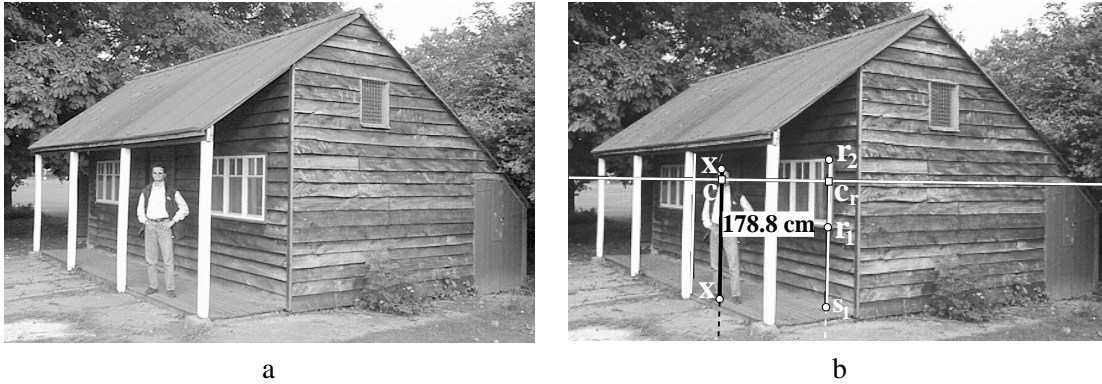
Figure 5.5: Measuring the height of a person from single view: (a) original image; (b) the height of the person is computed from the image as 178.8cm; the true height is 180cm, but note that the person is leaning down a bit on his right foot. The vanishing line is shown in white; the vertical vanishing point is not shown since it lies well below the image. The reference distance is in white (the height of the window frame on the right). Compare the marked points with the ones in fig. 5.4.
