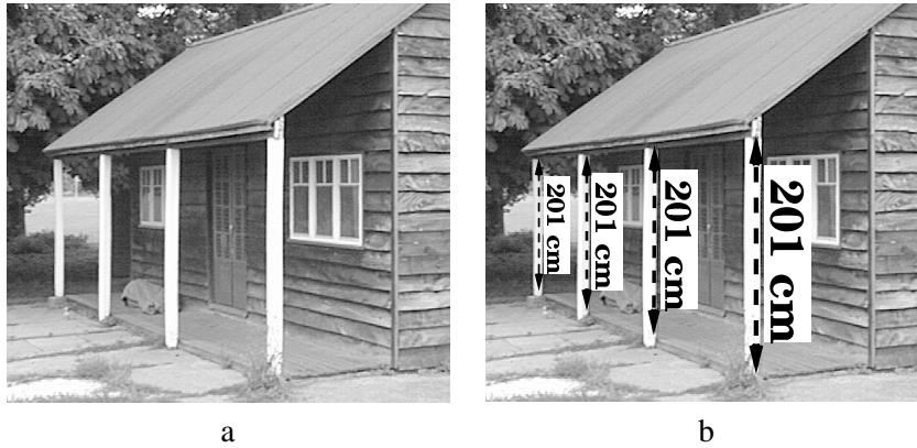
Figure 5.1: Measuring distances of points from a reference plane (the ground) in a single image: (a) the four pillars have the same height in the world, although their images clearly are not of the same length due to perspective effects; (b) as shown, however, all pillars are correctly measured to have the same height.
