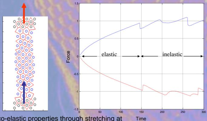
Visco-elastic properties through stretching at constant speed.
