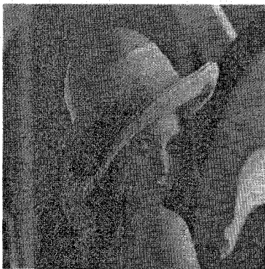
Figure 6. Lena compressed with recursive PVQ with quadtree at 0.33bpp; PSNR = 32.3 dB; Block sizes used in encoding: 2x2 up to 8x8
