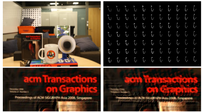
Figure 6: Visualization of ground-truth spatially-varying PSFs: For the blurry image on top, we show a sparsely sampled visualization of the blur kernels across the image plane. There is quite a significant variation across the image plane. To demonstrate the importance of accounting for spatially variance, in the bottom row we show a result where we have deconvolved using the PSF for the correct part of the image and a non-corresponding area.
