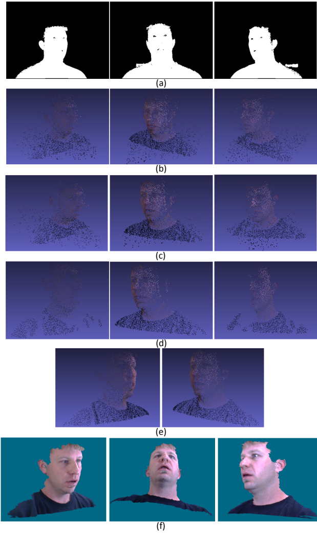
Fig. 6. Results illustrating different steps during sparse point cloud reconstruction. The input images were shown in Fig. 2 (b). (a) The IR masks. (b) Raw sparse point clouds of the three plan sweeping as shown in Fig. 5, without using collaborative filtering in score-volume. (c) Raw sparse point clouds of the three plan sweeping as shown in Fig. 5, using collaborative filtering in score-volume. (d) Post-filtered sparse point clouds. (e) Two views of the merged sparse point cloud. (f) Rendering results from various viewpoints based on the sparse cloud.
