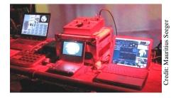
Figure 1: Typical VJ set up, showing laptops (running Resolume and Modul8 software), video mixer, monitor and other peripheral devices.
