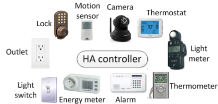
Figure 1: An example home automation system
