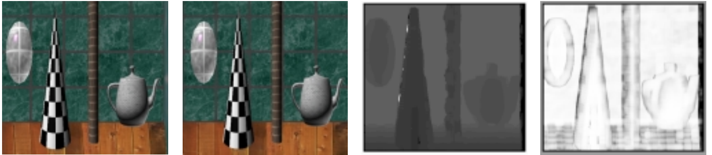
Fig.13 Parallel stereo with synthetic images: (a)(b) image pair; (c) result; (d) correlation map.
