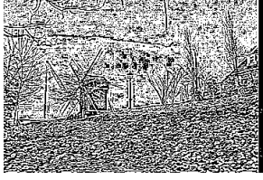
Fig. 7. The image of level 2 of the binary pyramid generated from the 2nd frame in the “Flowergarden” sequence.
