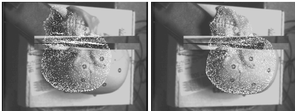
Figure 5.10: An image including an artificial occlusion. White spots denote the pose of the model. On the left is the initial pose, on the right is the final pose.
