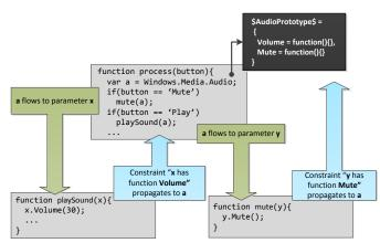
Fig. 3: Points-to flowing facts downwards and use analysis flowing data upwards.
