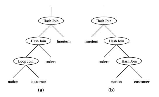
Figure 9: Plans chosen for Query 10 by (a) traditional statistics, and (b) sub-plan memoization
