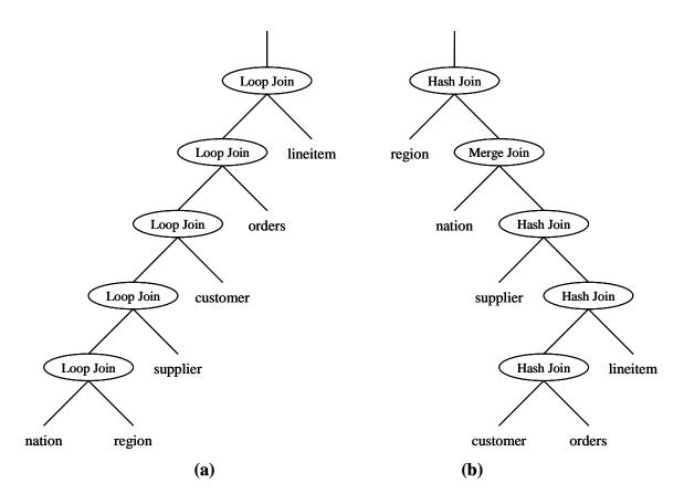
Figure 8: Plans chosen for Query 5 by (a) traditional statistics, and (b) sub-plan memoization
