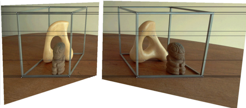
(c) Image pair transformed by the similarity \mathbf{H}_r and \mathbf{H}'_r . Note that the image pair is now rectified (the epipolar lines are horizontally aligned).
