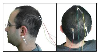
Figure 4. Electrode placement in our experimental setup.
