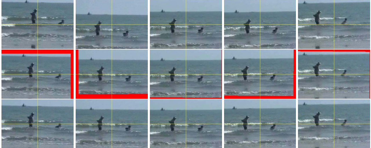
Figure 7: Result of video stabilization. Top row: Original input sequence, middle row: stabilized sequence which still has missing image areas, and bottom row: stabilized and completed sequence. The grid is overlaid for better visualization.
