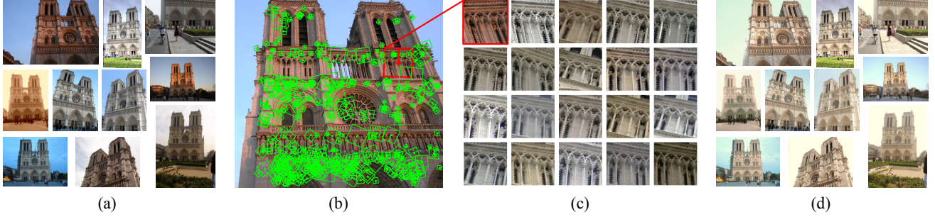
Figure 2. Overview: (a) Selected input images. (b) Keypoints extracted in an image. (c) Local feature descriptors are matched to obtain sets of aligned image patches from which the low-rank matrix is constructed. (d) We factorize this matrix using our robust technique and jointly estimate color correction parameters for each image. (d) The same set of images after color correction.
