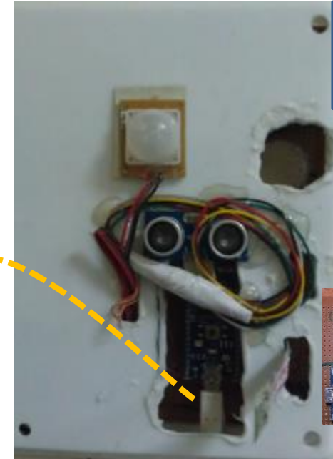
PIR, light, ultrasound, and temp sensors
