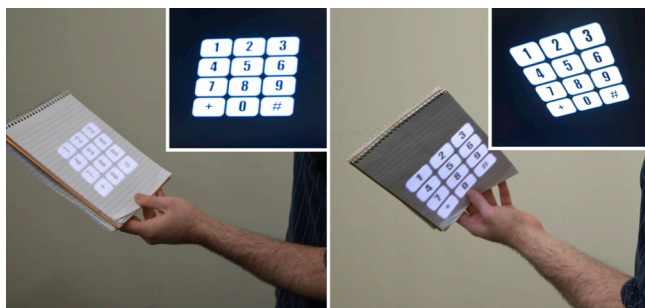
Figure 6. In order for interfaces to appear visually aligned and correct when projected onto moving surfaces, the projected image must be dynamically pre-distorted (see inset images).
