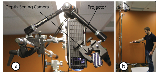
Figure 7. (a) LightGuide uses a single projector and depth sensing camera, (b) the projector and depth camera are fixed over the user's body.
