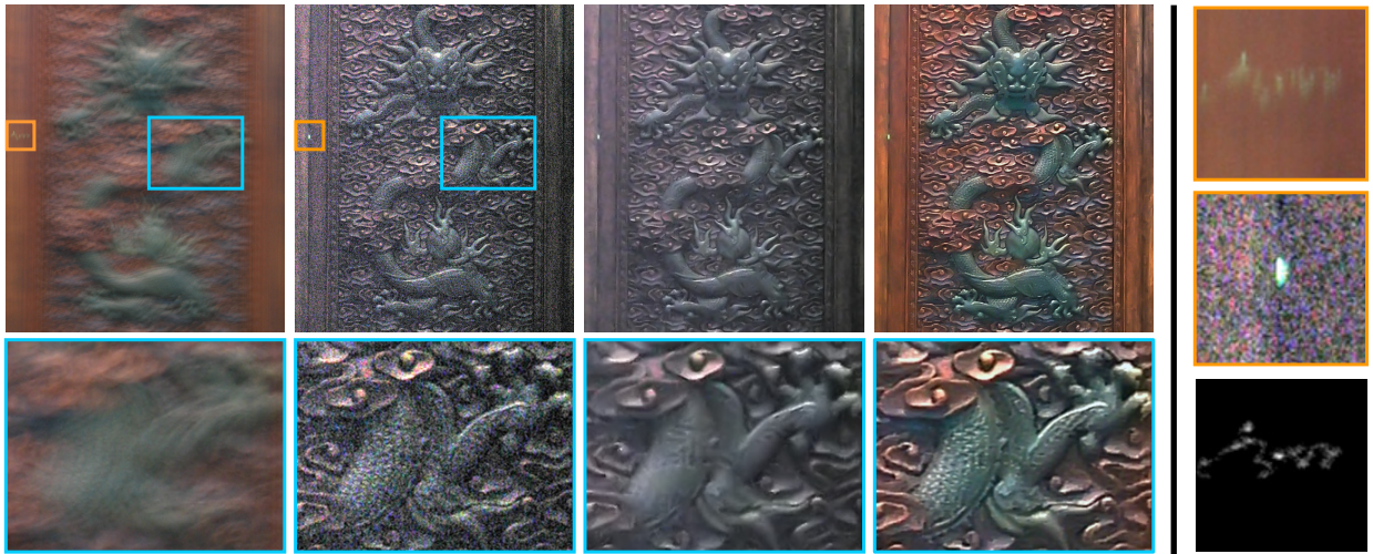
Figure 11: Large kernel. Left: blurred image, noisy image, denoised image, and our result. Top right: two image patches in the light-orange boxes in blurred/noisy images reveal the kernel shape. Note that the highlight point in the noisy patch is an ellipse-like shape. Bottom right: estimated 87 \times 87 kernel.
