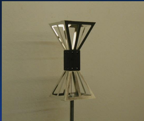
Outdoor omni-directional VHF/UHF antenna (flat 2 dBi gain over 150 – 1000 MHz)
