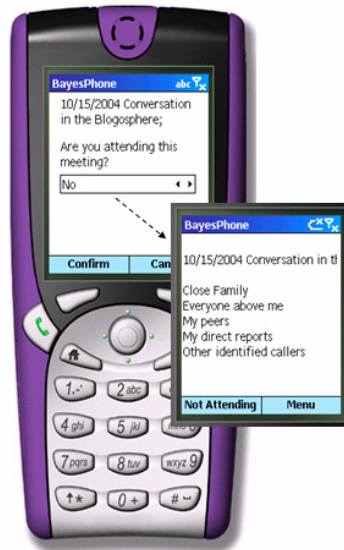
Fig. 5. Bayesphone application, showing the case where it is best to ask the user about attendance of a forthcoming meeting. When the meeting starts, the application displays the title of the meeting in progress, the input from the user, and the callers who can break through.
