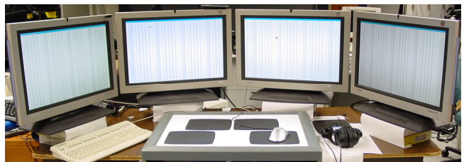
Figure 2: M^3 test setup consisting of four monitors and four corresponding “mouse pads” used by mouse location switch. The background is set to an inactive spreadsheet image to simulate a typical noisy working environment.
