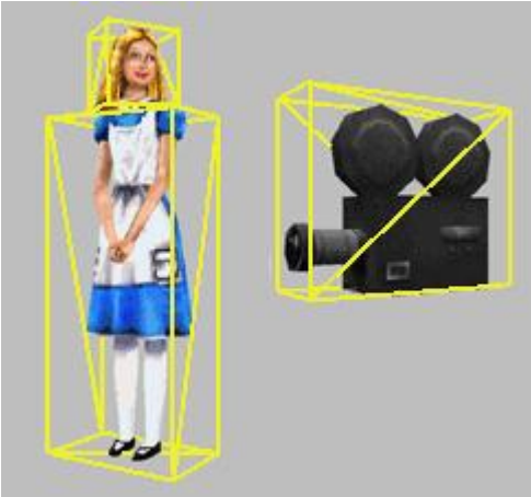
Figure 2: Immersive metaphor - head and body separation; Non-immersive metaphor - single camera
