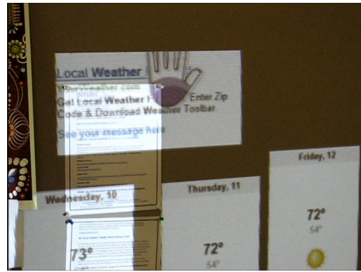
Fig. 7: SURROUNDWEB maps natural gestures to mouse events. Here, the user uses a standard “push” gesture to tell SURROUNDWEB to inject a click event into the web application.
