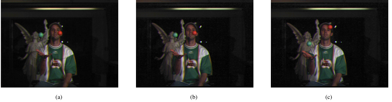
Figure 4: For synchronized cameras, the motion due to parallax between neighboring cameras is often much less than the temporal motion between frames for the same camera. (a) and (b) are images from adjacent cameras at the same point in time. Disparities between images are small. (c) shows a picture from the same camera as (b), one frame later. The motion is obvious and much larger.
