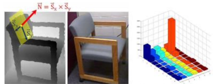
(a) Normal vector to represent tangent plane at (x, y, d(x, y)) .
