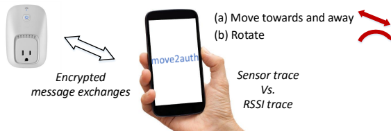
Fig. 2. Proximity based IoT device authentication. User holds smartphone and performs small gestures (a. move towards and away, b. rotate) in front of IoT device while IoT device is transmitting. Smartphone compares sensor trace with rssi trace to determine whether the device is in proximity.
