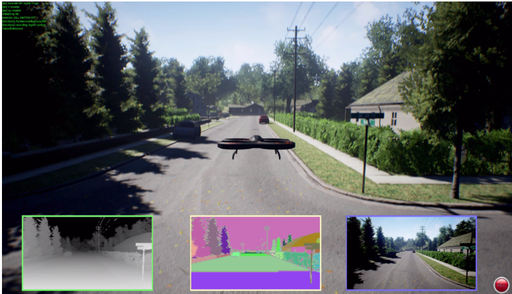
Figure 1: A snapshot from Aerial Informatics and Robotics Platform shows an urban environment in which a UAV is flying. The depth image stream, the materials property view stream and the front camera image stream are shown in real time in the inset.
