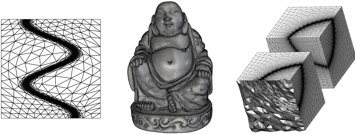
Figure 1: Anisotropic meshes generated by our method. Left: 2D meshing. The anisotropic metric is defined as the Hessian of an analytic function evincing a large range of anisotropy ratios ( \lambda \in [1.9, 394.4] ). Zoom in on the image to see meshing details. Middle: 3D surface meshing of the Happy Buddha from curvature tensors estimated from a high-resolution reference mesh (115474 vertices). Our relaxation produces a high quality result (63284 vertices) starting with an initial low-resolution mesh (5000 vertices). Right: volumetric meshing in a 3D cube. Anisotropy changes substantially ( \lambda \in [1, 40] ) and rapidly over the domain. The lower image shows a cross-section.
