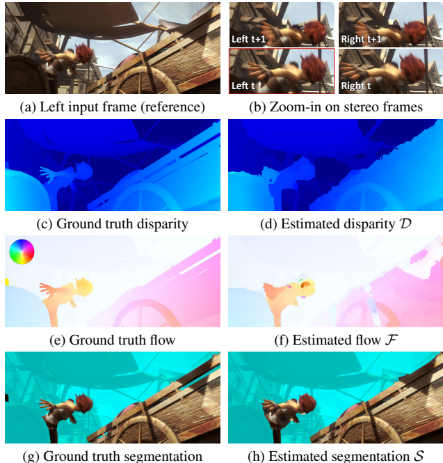
Figure 1. Our method estimates dense disparity and optical flow from stereo pairs, which is equivalent to stereoscopic scene flow estimation. The camera motion is simultaneously recovered and allows moving objects to be explicitly segmented in our approach.
