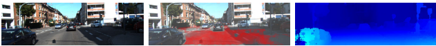
Figure 6. Segmentation ground prior. For road scenes (left), we compute the ground prior (middle) from the disparity map (right).
