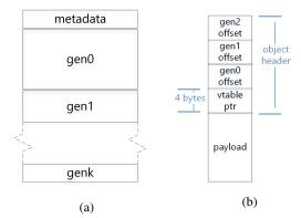
Figure 1: (a) Layout of a segment and (b) layout of a gen3 object in our allocator. The header contains the segment-relative offsets of incarnations of this object in all lower generations.
