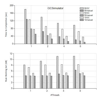
Figure 6: Time to completion and peak working set of the GC simulator benchmark with garbage collection and manual memory management with varying number of threads and percentage of short lived objects.
