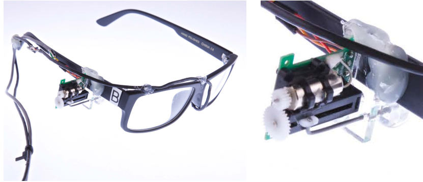
Fig. 5. Glasses with a linear actuator for tapping. The whole frame is shown on the left. A close-up of the linear servo is shown on the right.
